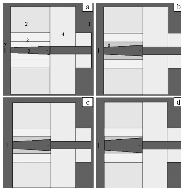
Fig. 4. The MCNP5 geometries and materials of collimator parts; 1 – air, 2 – concrete, 3 – iron, 4 – polyethylene, 5 – air cone, 6 – lead metal, 7 – beryllium target
